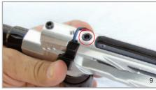
Remove Ram Sleeve Retaining Allen
