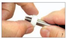
Remove Delrin Bolt Pin Receiver Spacer
