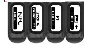
From the Run Screen push and hold the <sup>®</sup> button. Initially, the current Preset configuration will be displayed and then after one 1 second **OFF?** will be displayed, the first item on the Main Menu.
