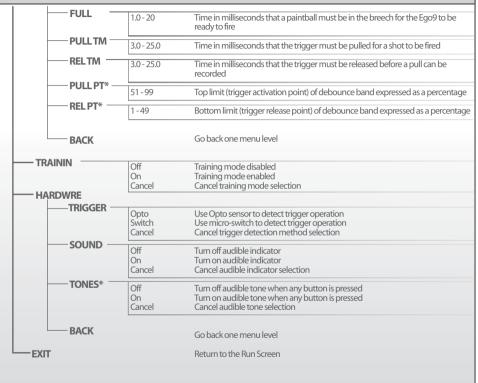
Parameters followed by a \* are part of the smart menu system and will only be displayed depending on your chosen settings. (E.g. The MAX ROF parameter will only become available if the ROF CAP parameter is set to on).
