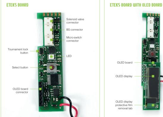
ETEKS BOARD WITH OLED BOARD FITTED
