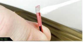
Remove the rubber detent and using a dry cotton bud clean the detent and its location point in the GSL body, replacing the detent if it is damaged (SEE FIGURE 15D).
