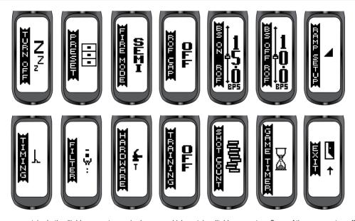
The Main menu contains both editable parameters and sub-menus which contain editable parameters. Some of these parameters affect the way the GSL shoots and are tournament locked as standard from the factory.1
