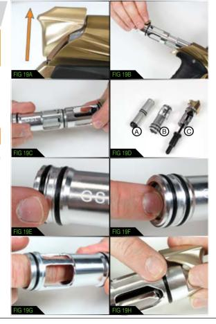
Take the bolt and having cleaned off any old grease, paint or debris, examine the rubber bolt tip for any signs of damage (SEE FIGURE 19J), replacing if necessary.
