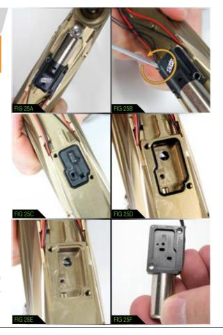
Check the underside of the solenoid valve to ensure that it is free from damage or debris (SEE FIGURE 25F).
