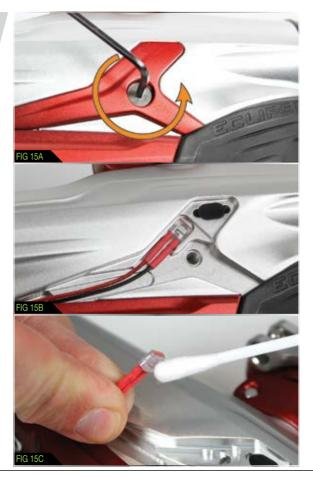
Remove the rubber detent and using a dry cotton bud clean the detent and its location point in the GEO3.1 body, replacing the detent if it is damaged (SEE FIGURE 15D).
