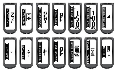
The Main menu contains both editable parameters and sub-menus which contain editable parameters. Some of these parameters affect the way the GEO3.1 shoots and are tournament locked as standard from the factory.1
