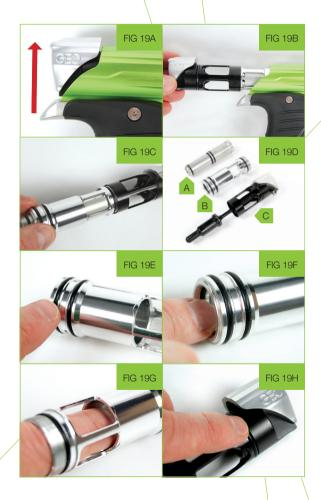
Smear a light coat of Eclipse Grease onto the smooth internal bore of the bolt can from the rear (see figure 19G).
