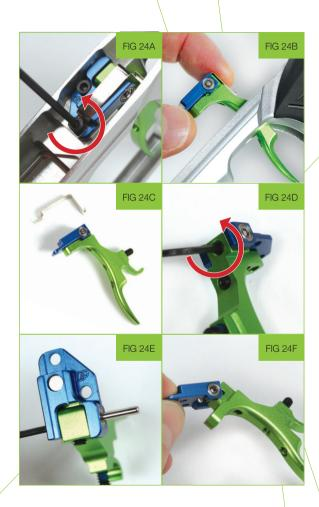
Position the trigger so that the hole through the trigger lines up with the holes in the bearing carrier, slide the trigger pin into place (see figure 24G).
