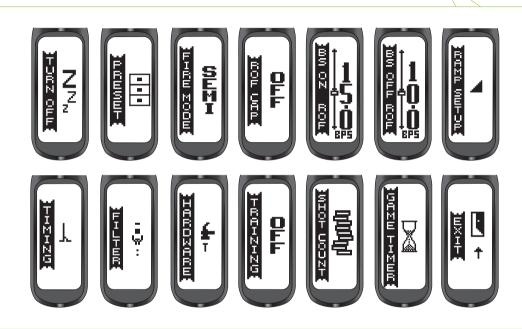
The Main menu contains both editable parameters and sub-menus which contain editable parameters. Some of these parameters affect the way the GEO3.5 shoots and are tournament locked as standard from the factory.<sup>1</sup>
