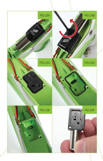
Check the underside of the solenoid valve to ensure that it is free from damage or debris (see figure 25F).
