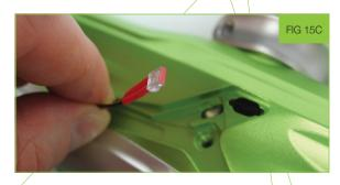
Remove the rubber detent and using a dry cotton bud clean the detent and its location point in the GEO3.5 body, replacing the detent if it is damaged (see figure 15D)
