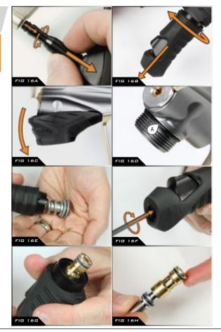
At this point if you are maintaining the inline regulator to fix a supercharging issue, turn to page 46 to the 'ADVANCED SL4 INLINE REGULATOR MAINTENANCE' section. If you are not fixing a supercharging issue then there is no need to perform this advanced maintenance procedure.
