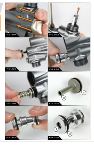
Screw the LPR adjuster out from the LPR cap using a 1/8" hex key (SEE FIGURE 201). Clean and inspect the adjuster o-ring (LABELLED & FIGURE 201), replacing if necessary. Lubricate the o-ring with a small amount of grease.
