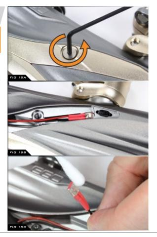
Remove the rubber Detent and using a dry cotton bud clean the Detent and its location point in the Ego LV1 body, replacing the Detent if it is damaged (SEE FIGURE 15D).
