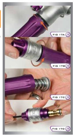
Using a dry cotton bud, clean the internal 008 NBR70 o-ring that sits inside the top section of the adjuster top. Then using a small hex key gently apply Eclipse Grease to the o-ring (See Figure 1.75).<sup>1</sup>
