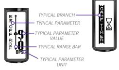
On parameter screens a range bar will be displayed where there is a large scale of adjustability in that parameter. The current parameter value is displayed as a box on the range bar which is used to indicate the range of adjustability in the parameter value.
