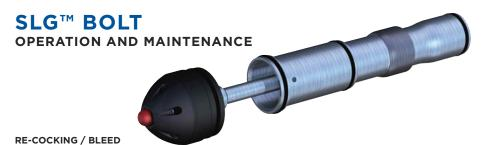
The  $SLG^{\text{TM}}$  is equipped with a Pneumatic re-cocking system in case the bolt becomes jammed (pinching a ball). The button in the center of the bolt back can be pressed to send the bolt rearward and reset it for the next shot. The bleed button also serves as a gas vent for the dump chamber. It can be used to de-gas the  $SLG^{\text{TM}}$  after the tank is removed, or to confirm that the  $SLG^{\text{TM}}$  has gas and is ready for play.
