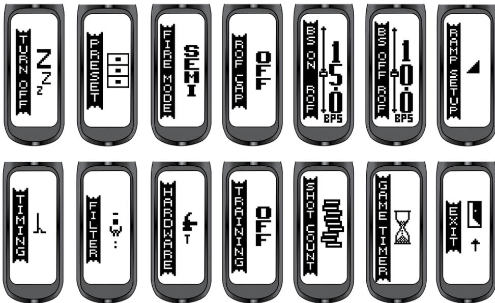
The Main menu contains both editable parameters and sub-menus which contain editable parameters. Some of these parameters affect the way the Ego LV1 shoots and are tournament locked as standard from the factory.<sup>1</sup>
